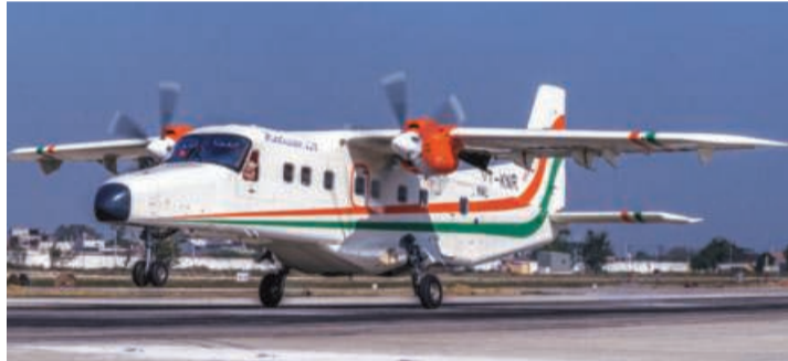
The Hindustan-228 aircraft is a multi-purpose, light-weight, twin turboprop aircraft. It has been indigenised by HAL to operate on short haul air routes under the regional connectivity scheme UDAN
